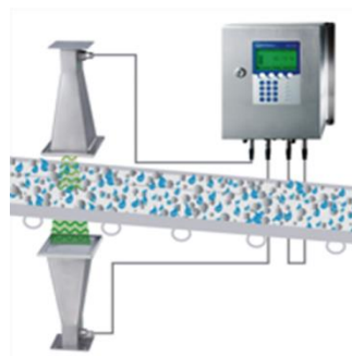
Fig 1. Soil moisture measurement system using antenna
